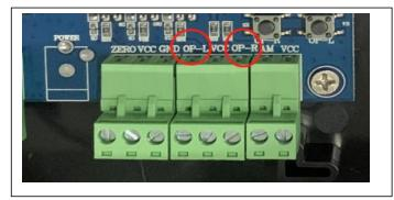
220V power to air switch , either port is ok
